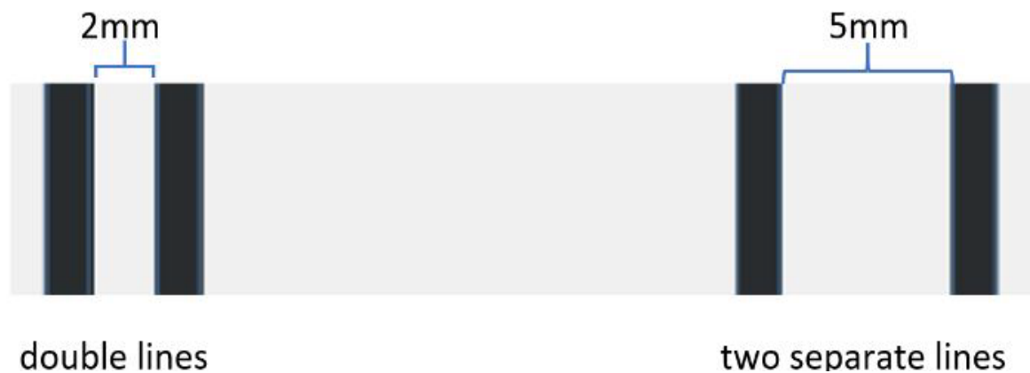
Figure 5g: Use a minimum distance of 2mm between double lines and 5mm between separate lines. Original image.
