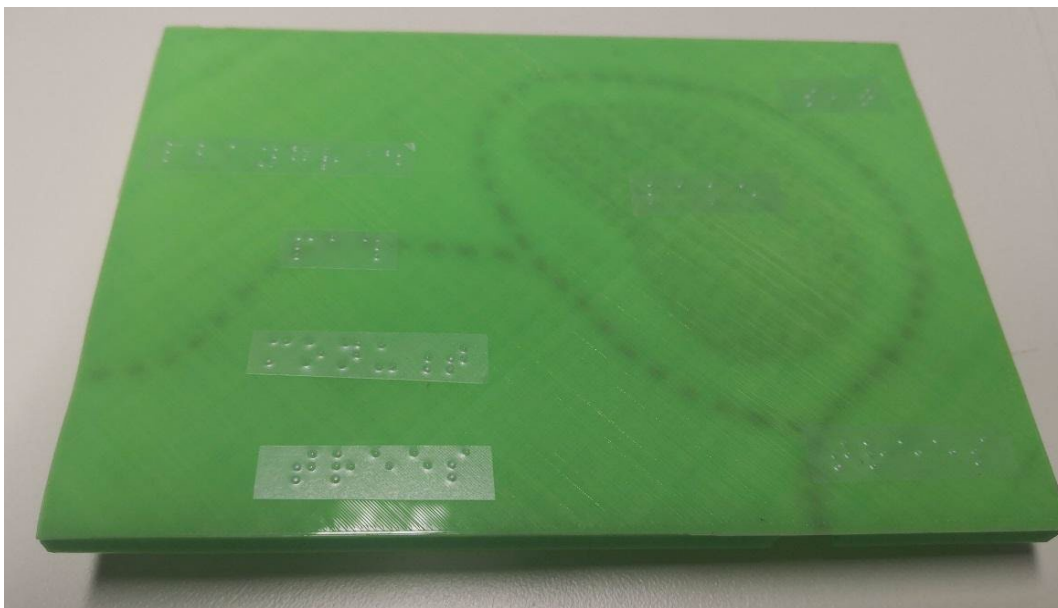
Figure 8d: Sticky braille labels placed under key features on a flat-based 3D model. Image courtesy of Monash University.
