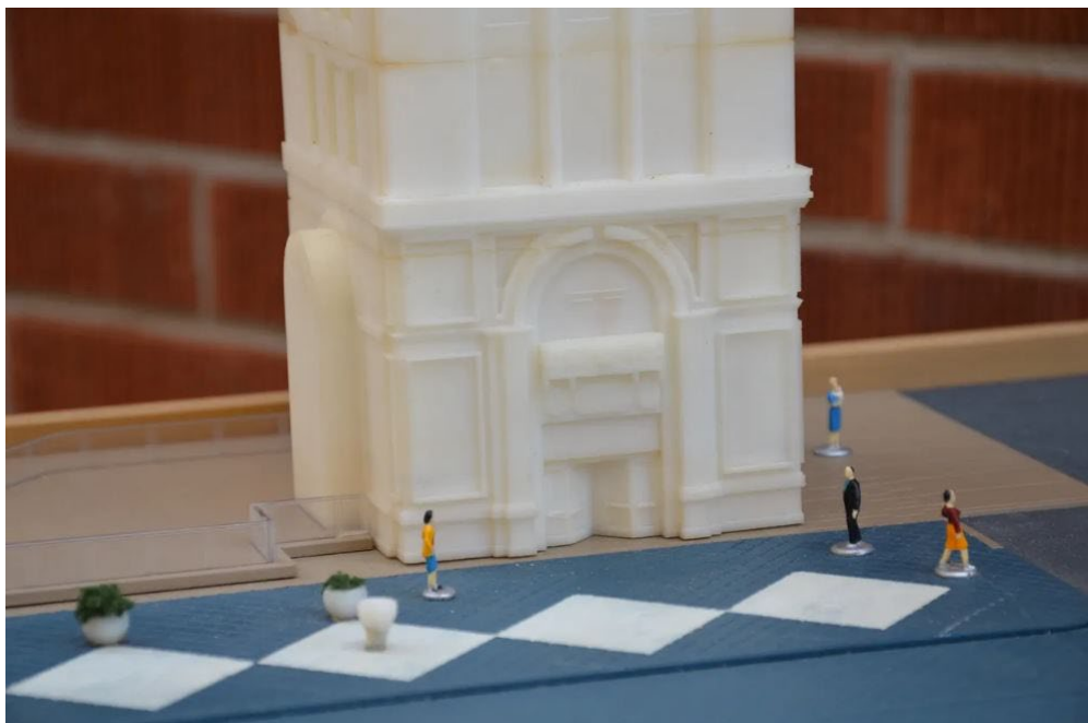
Figure 5e: Provide figures or other well-known objects alongside a 3D printed model of a real object to indicate scale. Image courtesy of Matthew Gesualdi, Tact-Ed.
