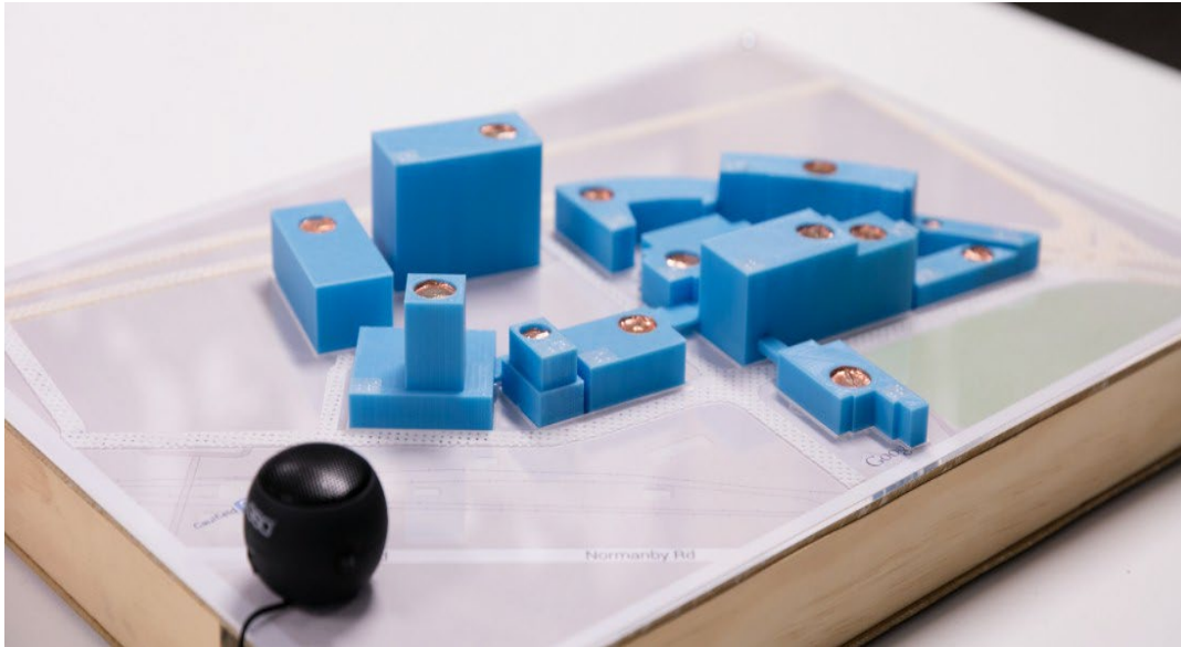
Figure 7b: Laser cut box as a base for 3D printed buildings, with etching to indicate roads and a box to house electronic components. Image courtesy of SensiLab, Monash University.
